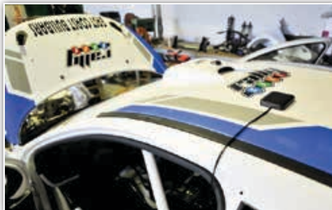
Stick-on Antenna is mounted on the ROOF of the vehicle, preferably within easy cable reach of the final RS unit mounting position allowing the cabling to then pass through the door seal and follow the cage bars back to the RS unit location.
